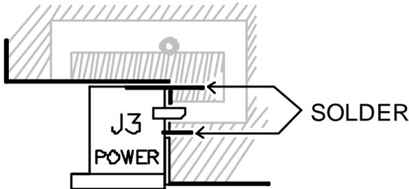
side. Do a trial positioning in order to understand how the jack is connected. Notice that the edges of the two jack lugs will be perpendicular to the PC board surface.
