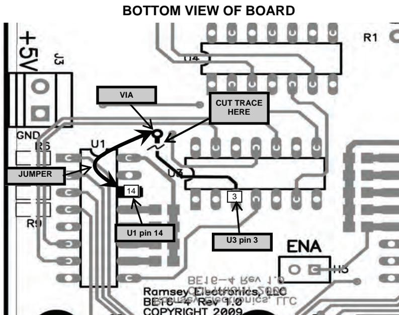
The operation of the BE164 with the DVMS8 system is as described below with the exception that only the first 8 input lines and only 3 output lines are used. By performing this modification to the BE164, only the first 8 input lines will activate J5 pin 2 and the signal becomes an active low signal used to activate the play function on the DVMS8. Once the units are interconnected simply taking an input line low will select the desired DVMS8 message and it will start playing.
