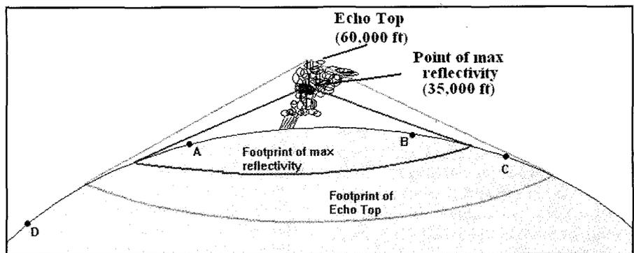
Figure 15. Footprint of a supercell thunderstorm with echo tops at 60,000 ft.
