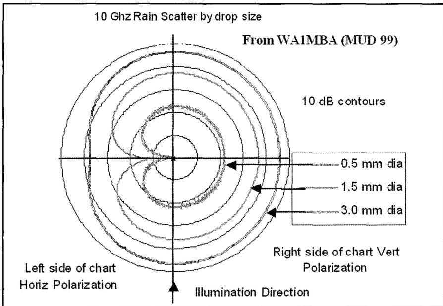
Figure 5. Scattering from spherical water droplets of different diameters at 10 GHz (from WA1MBA's presentation, MUD 99). Notice the large null at 90° with horizontal polarization.
