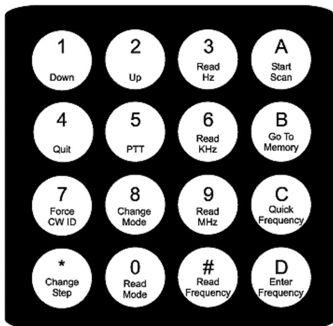
**Figure 1—Remote control commands issued via the DTMF keypad.**
