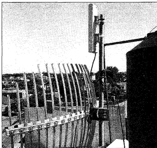
The Ubiquiti NanoStation transceiver in this photo is the white module just above the parabolic dish antenna. At 3.5 GHz, these inexpensive units have potential for amateur HSMM applications.
