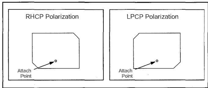
Figure 4. Left- and right-hand circular-polarized notches.
